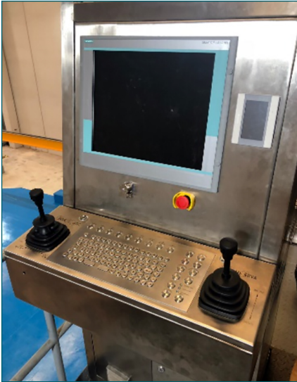
Figure 13. Manipulator console (mock-up).
