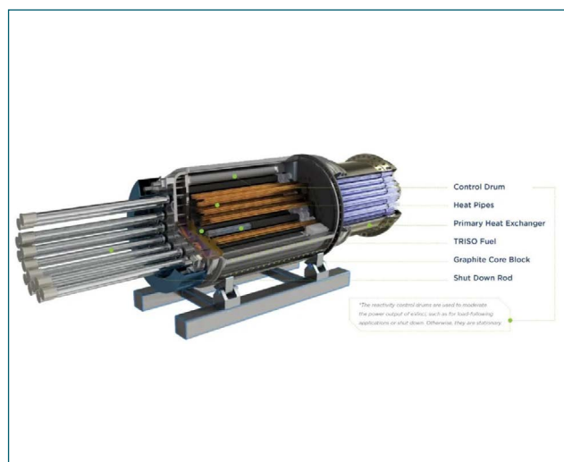
Figure 1. Conceptual design of the eVinci microreactor.
