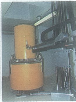
NUSTATION Radiation/contamination measuring station.
