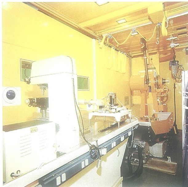
Instrumented system for Impact Testing, Fractographic Observation and Hardness
