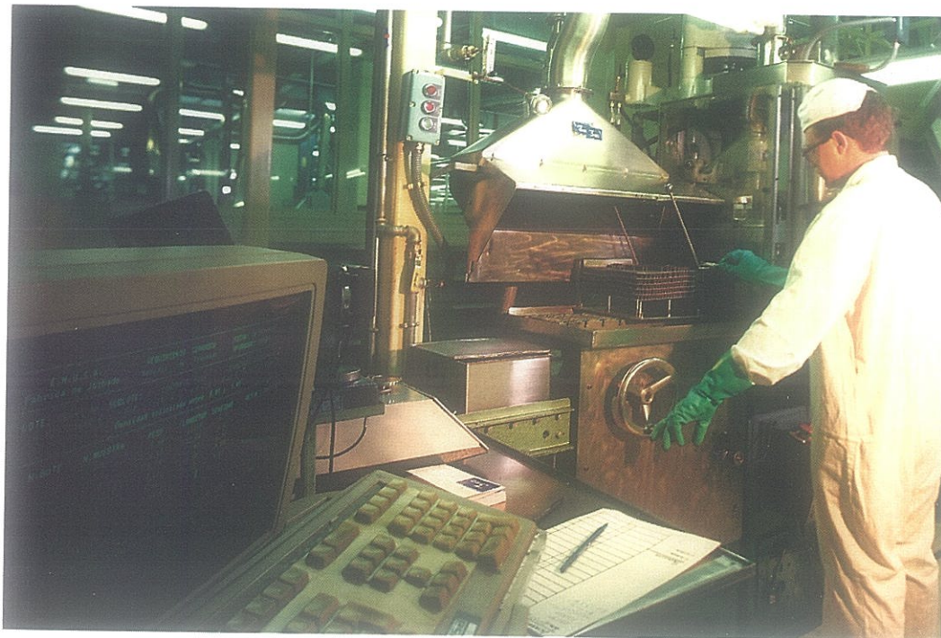
Gamma scanner for uranium oxide enrichment control (Juzbado Factory)
