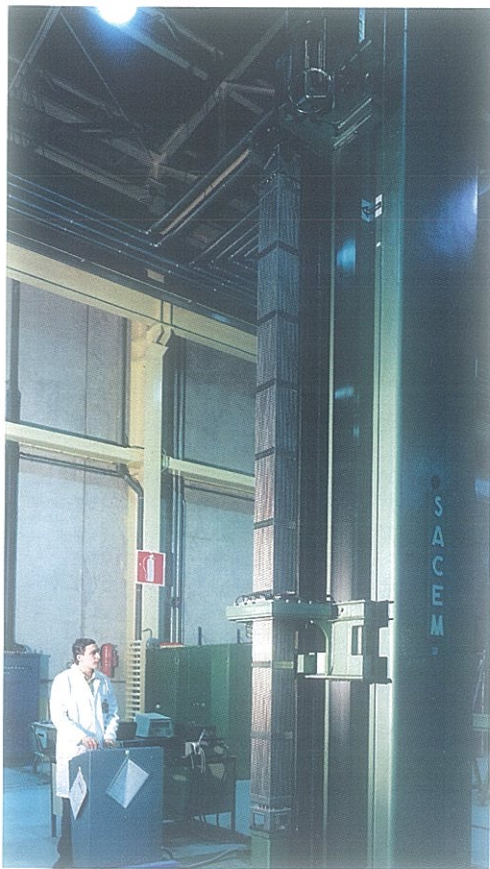
Final inspection of an XL fuel assembly for the European market.
