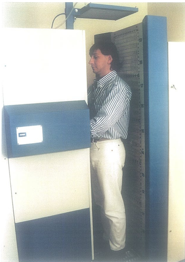
Whole body counter to detect incorporation of radionuclides
