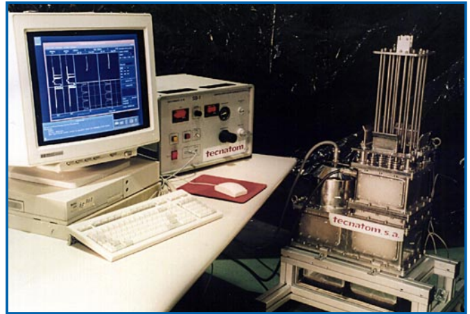
FV - Eddy-current control rod inspection system.
