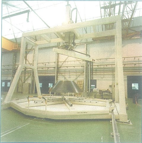
Figure 6: SICCO Inspection System
