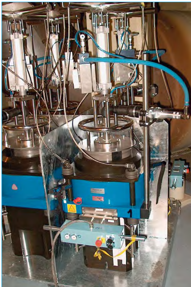
Reactor vessel closure Studs Tensioner.
