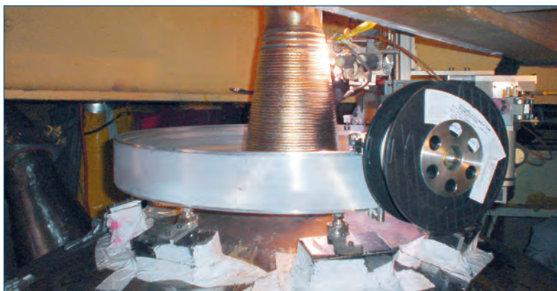
Figura 3. /Figure 3: Detalle cordones en tobera spray / Detail spray nozzle cords.
