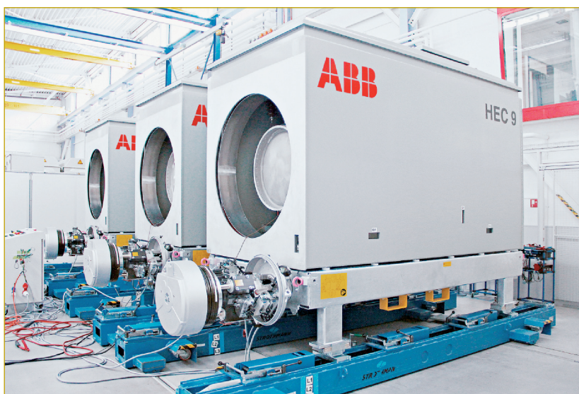
Figure 2. View of the three poles of the generator circuit-breaker system HEC 9.
