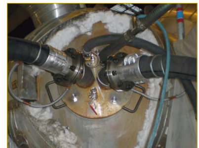
Sealing tool of the MSR water box.
