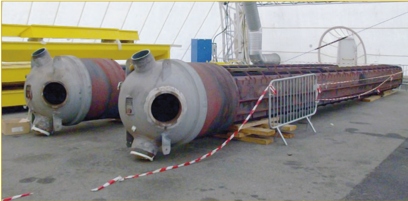
MSR tube bundles in workshop for the LMQ process homologation.
