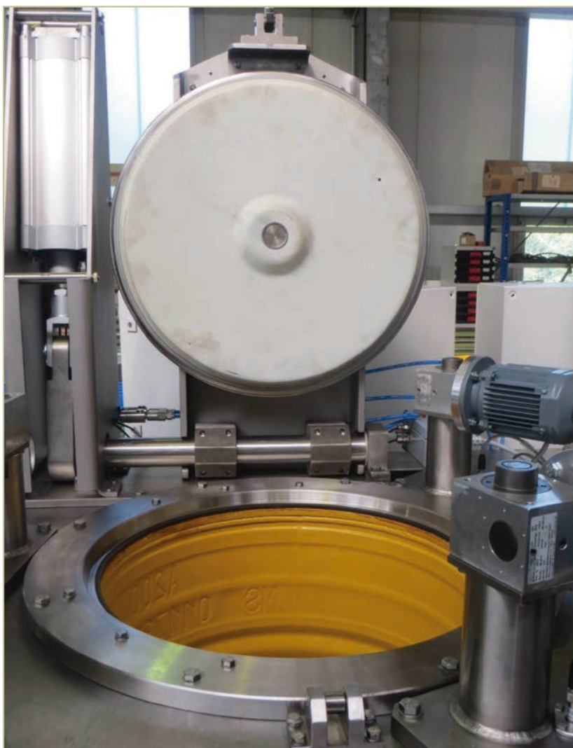
Figure 3: Double - lid Transfer Lock.
