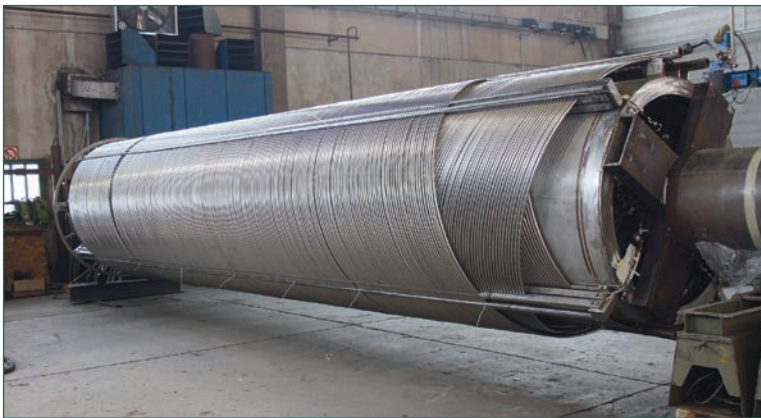
Figure 4. Section of full-scale steam generator assembly being prepared for testing in Italy.
