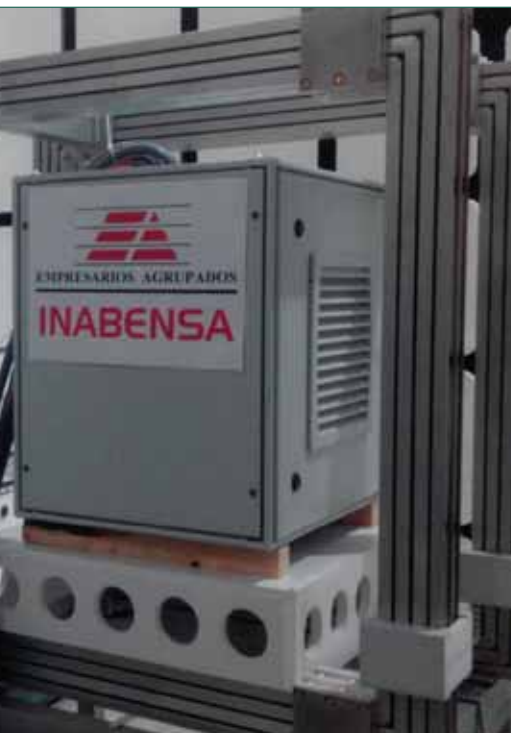
Figure 2. Dummy cubicle inside the static magnetic field induction coil.
