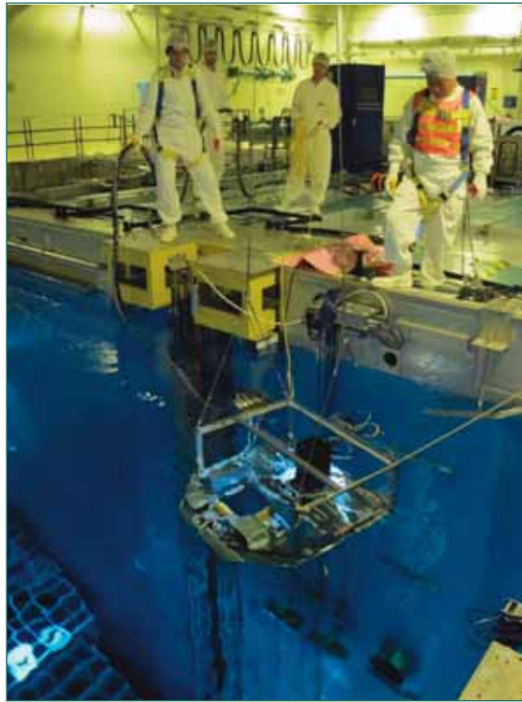
Figure 4. First introduction of the SICOM-COR into the spent fuel pool.
