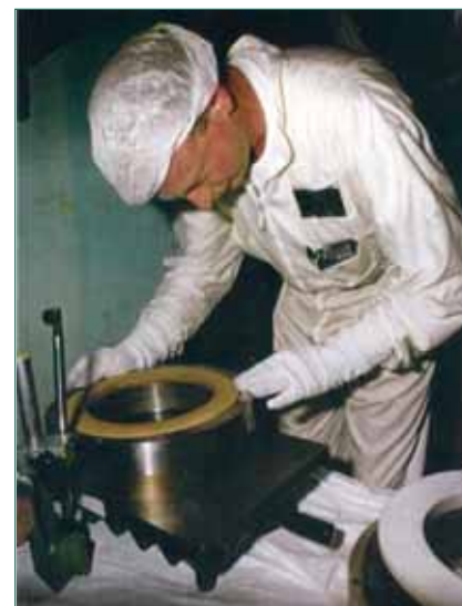
Figure 4. AREVA inspector working on a RCP seal.
