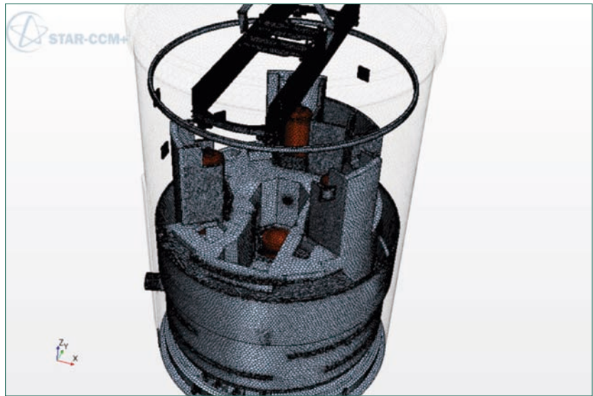
Figure 7. Reactor Building mesh overview.
