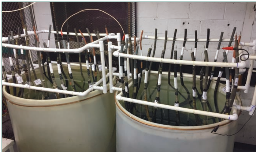
Figure 4. EPRI research being done to evaluate the effects of high-potential testing on commonly used cables.
