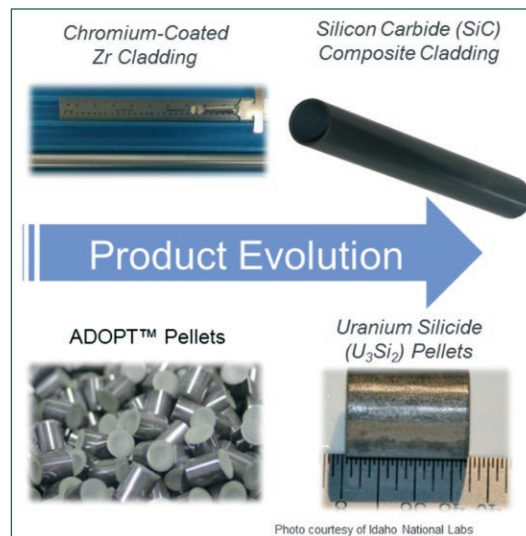
Figure 1. Fuel concepts considered in the Westinghouse EnCore® Fuel.
